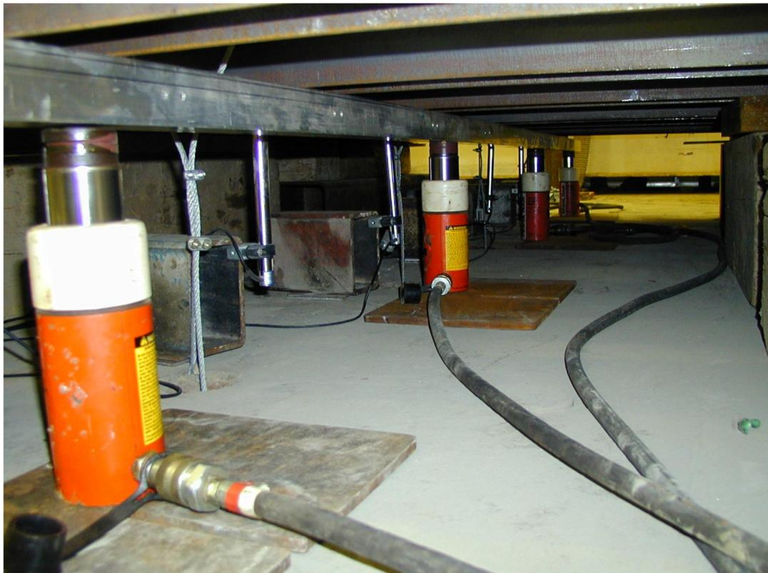
Figure 2. Hydraulic jack arrangement providing control for deflection testing.
