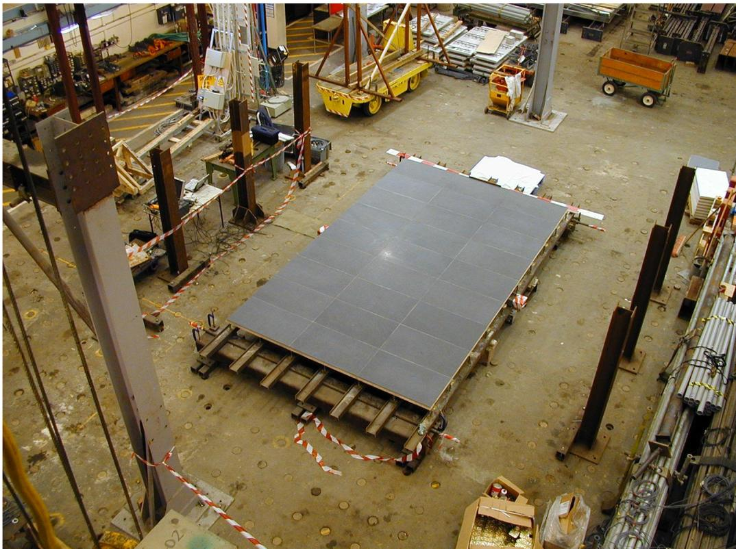
Figure 1. General view of floor constructed for deflection and rolling load testing at BRE.
