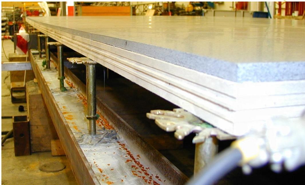
Figure 3. General view of floor panel system, sitting on pedestals for test.
